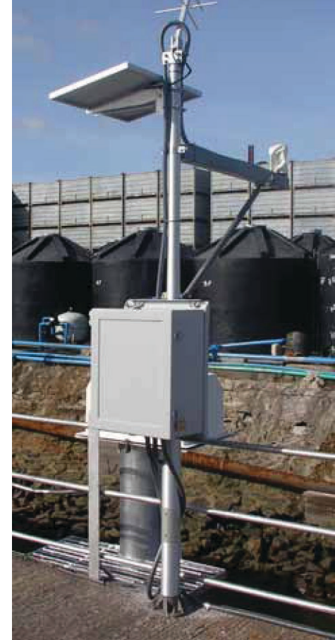
Figure 2. Sea Observations – A GLOSS tide gauge station at Lamu.
