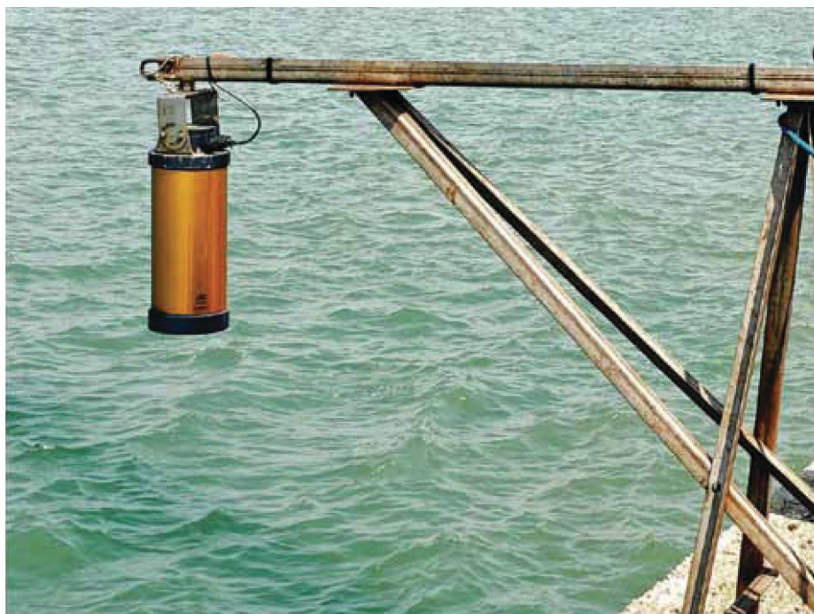
Figure 1. Tide gauge installed by ODINAFRICA at Pointe Noire port.
