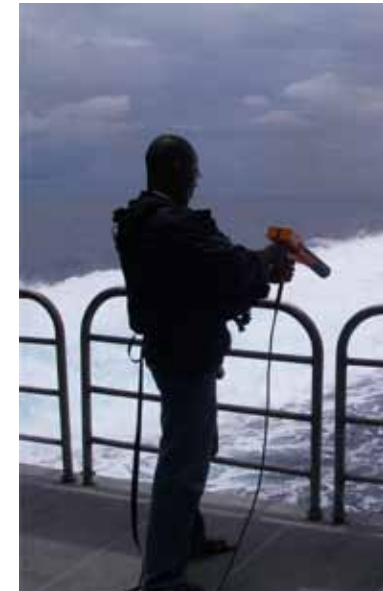
Figure 4. XBT (left) being shot into the sea off the Ghana coast (right).
